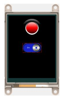
The Switch widget can be modified as needed through the **Object Inspector**.
